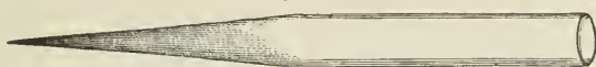
Portion of tube separated with a deposit of Metallic Arsenic in the contracted portion.
